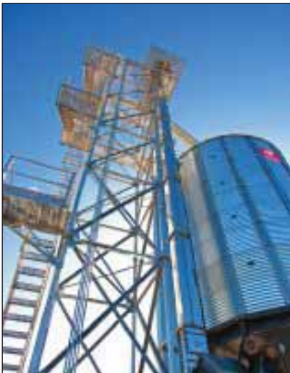
Incoming wet corn travels up a Chief 15,000-bph receiving leg supported by a Chief tower.
