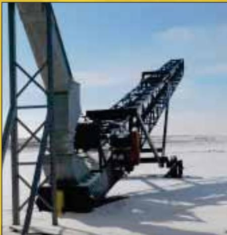
Gravity spout leading to a portable belt conveyor used for building emergency storage piles during harvest as needed.
